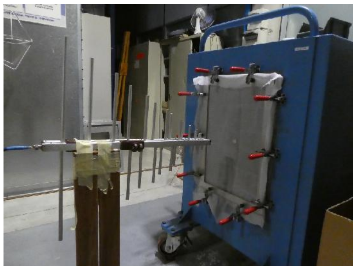
Picture 4: Electric field (300 MHz – 900 MHz) measurement test set-up on AC082522/1
