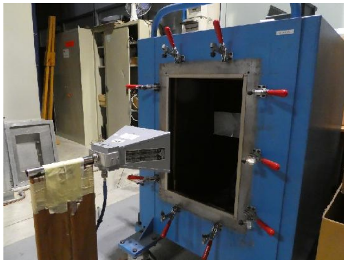
Picture 5: Electric field (1.6 GHz – 18 GHz) reference measurement test set-up
