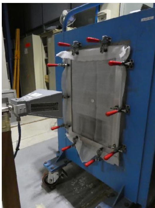
Picture 6: Electric field (1.6 GHz – 18 GHz) measurement test set-up on AC082522/1
